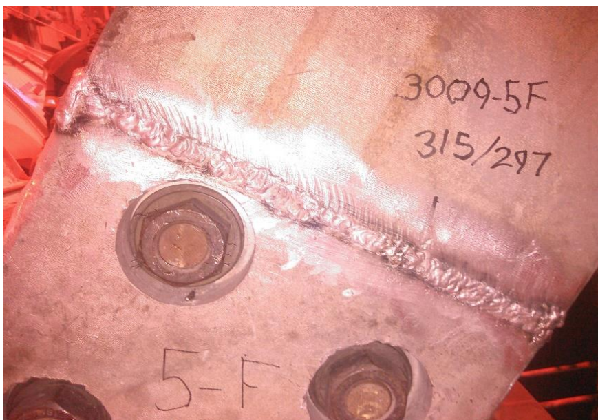
Figure 6. Example of good weld quality using the magnetic field attenuation.
